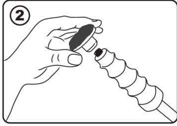
Take the suitable aluminum adaptor out of the box, identify the dent area also clean up the work surface. (4 sizes of aluminum adaptor available for selection)
