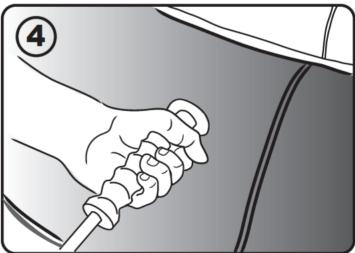
After the glue fixed on the adaptor, screw the aluminum adaptor on the sliding hammer.
